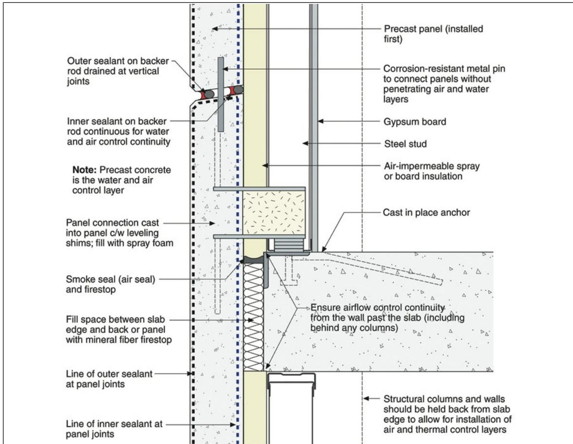
Figure 11: Section at floor of a high-performance architectural precast panel (CPCI 2013).
