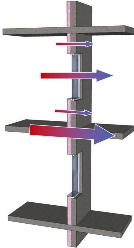
*Figure 4: Heat flow paths through centre of wall, floor slab, and windows (arrow size is relative to magnitude of heat flow).*
