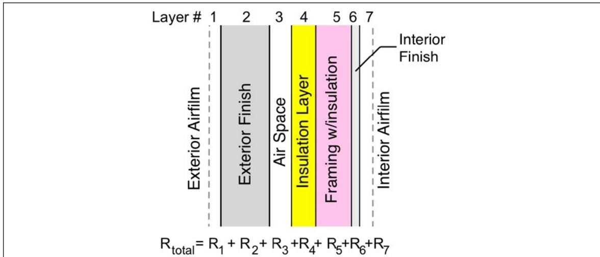
Figure 7: Example calculation of multi-layer assembly thermal resistance.
