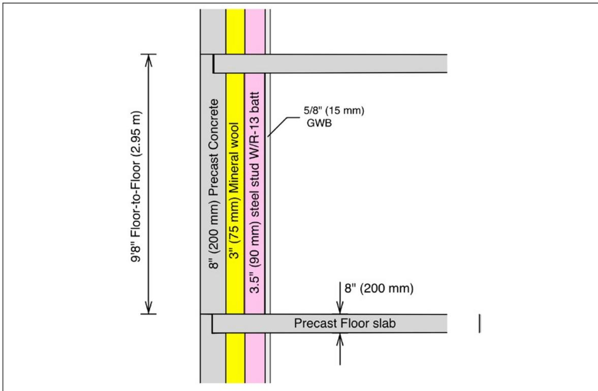
Figure 18: Example generic total precast whole wall.
