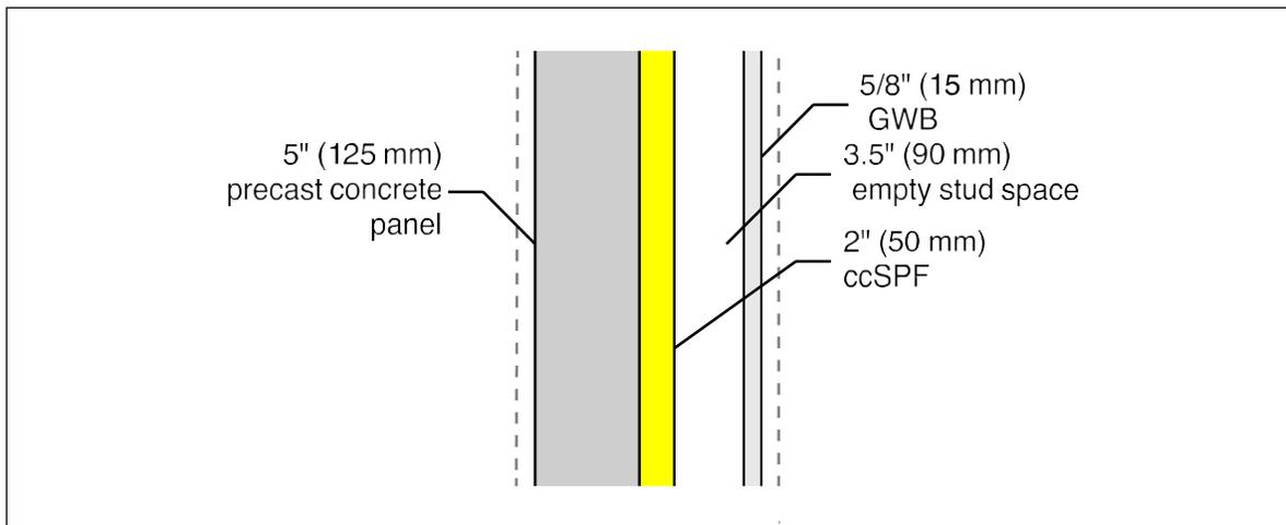
Figure 13: Example architectural precast assembly.
