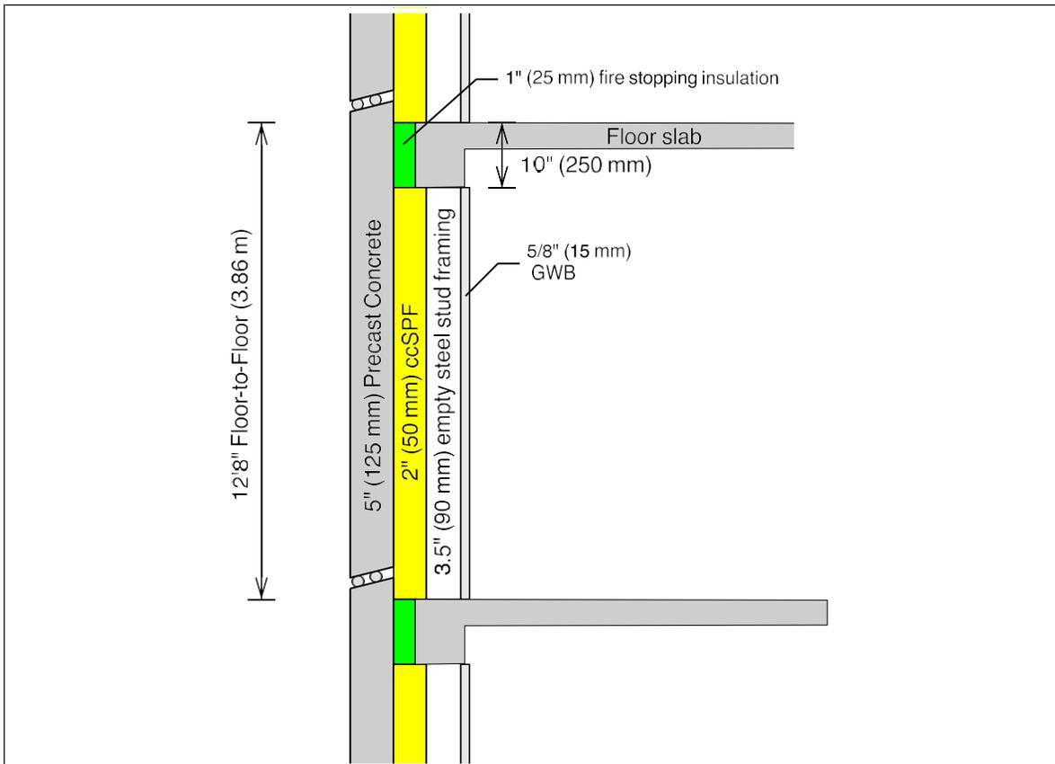
Figure 14: Example architectural precast system.
