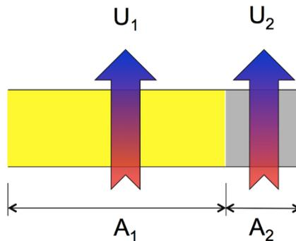
Figure 8: Parallel path heat flow.
