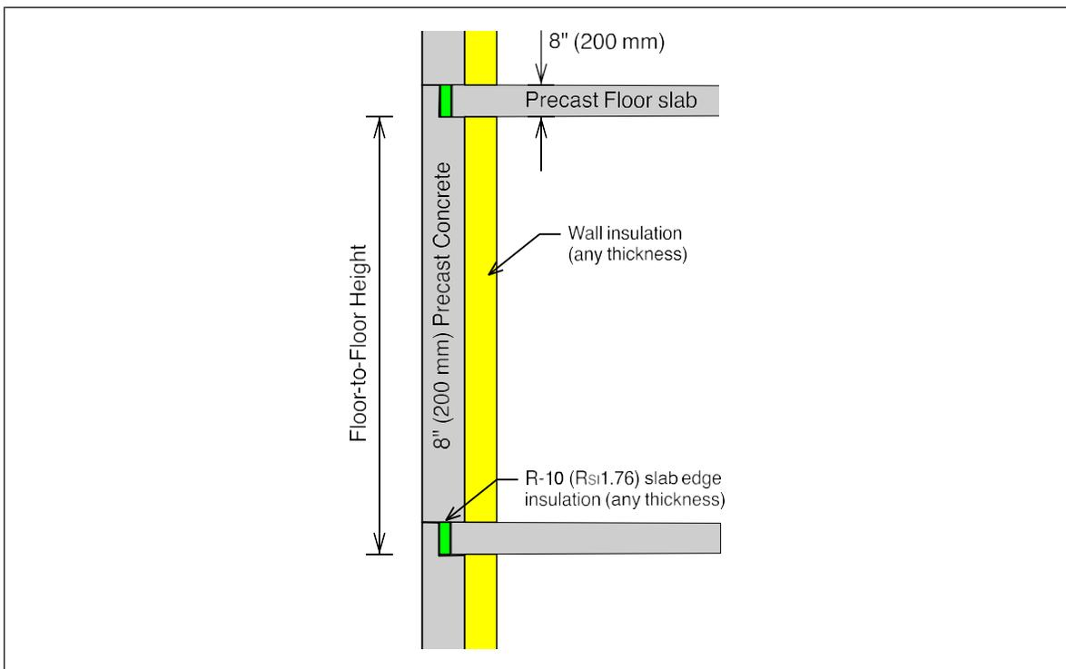
*Figure 19: Single-wythe total precast system with slab edge insulation assumed for calculations in Table 14.*
