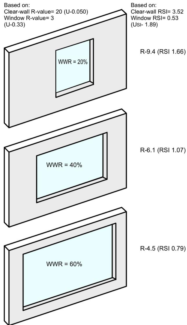
Figure 9: Impact of windows on overall enclosure R-value.
