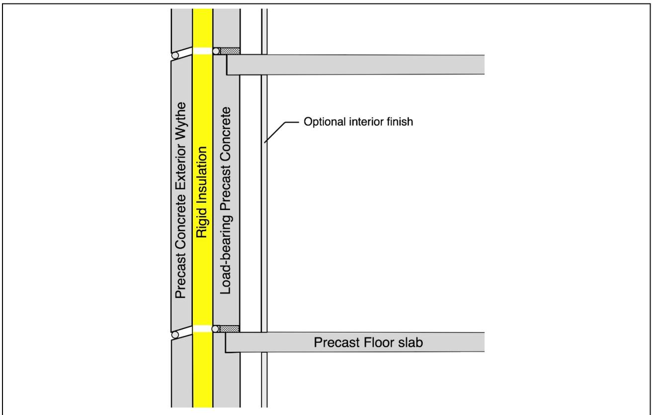
Figure 17: Double-wythe insulated “sandwich” total precast.
