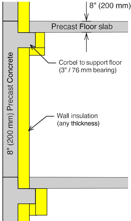
*Figure E1: Alternate insulated slab edge solution.*
