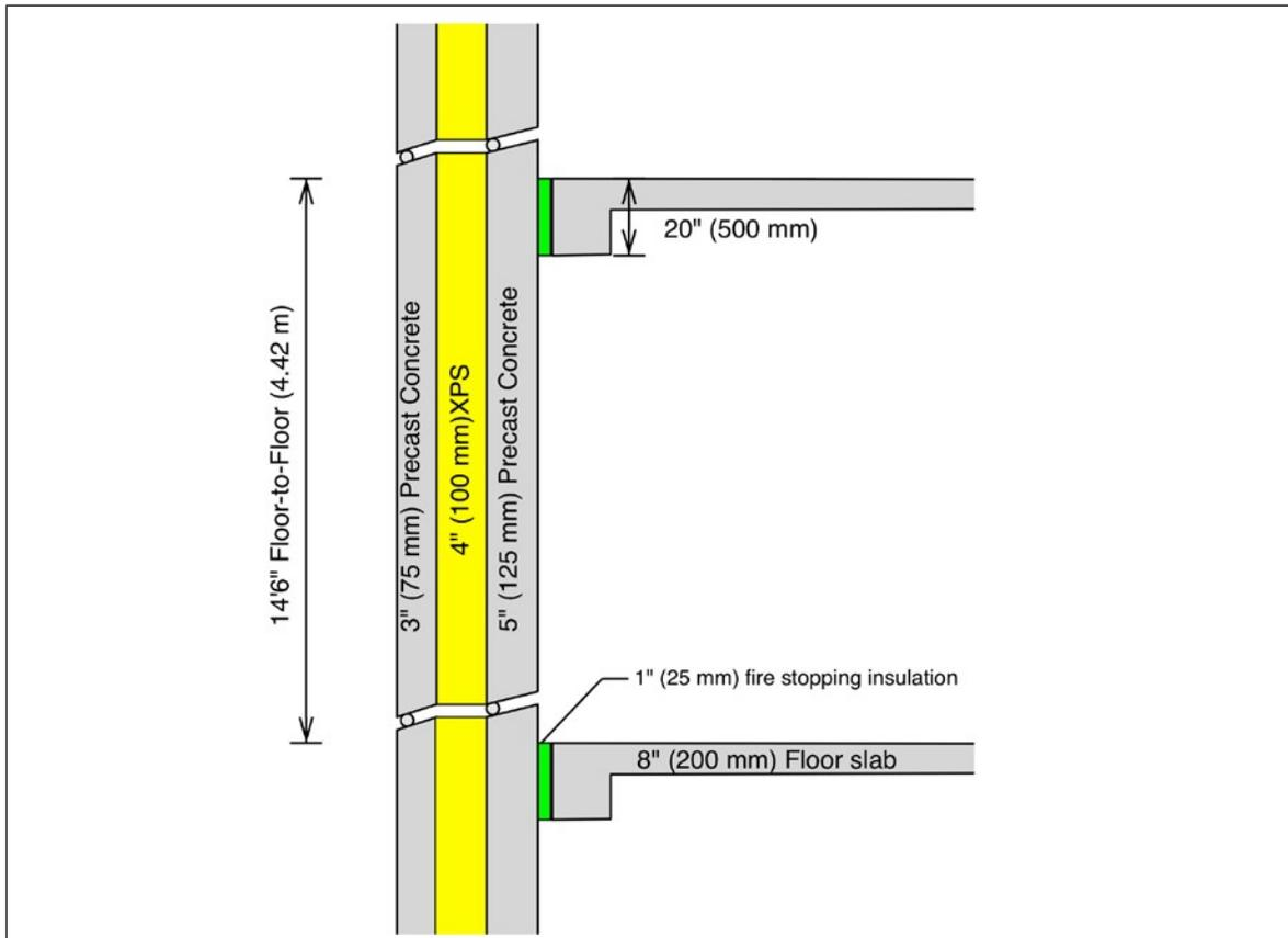
Figure 16: Example double-wythe (sandwich) panel.
