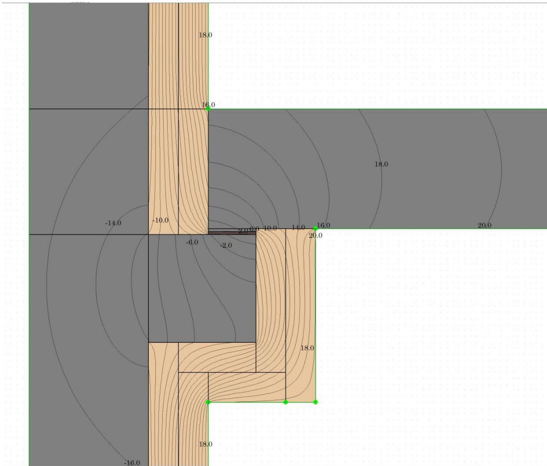
*Figure E2: Example of insulated corbel total precast system geometry and isotherms.*
