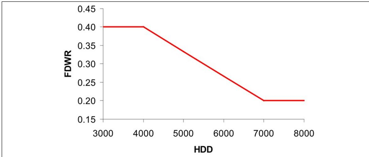
*Figure 3: Maximum fenestration-and-door-to-wall ratio (FDWR) under the NECB prescriptive approach.*
