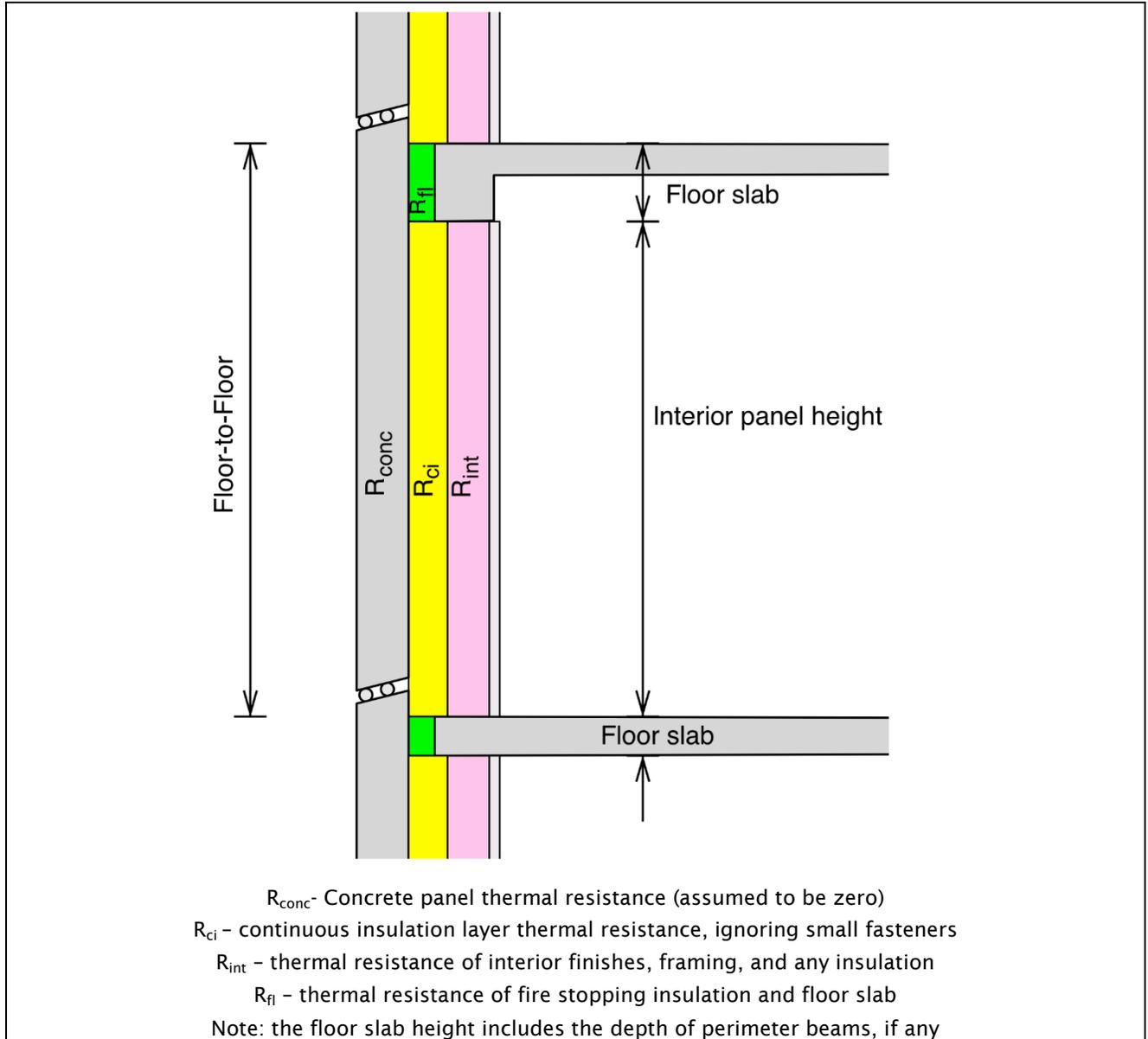
Figure 12: Definition of terms for architectural precast thermal calculation.
