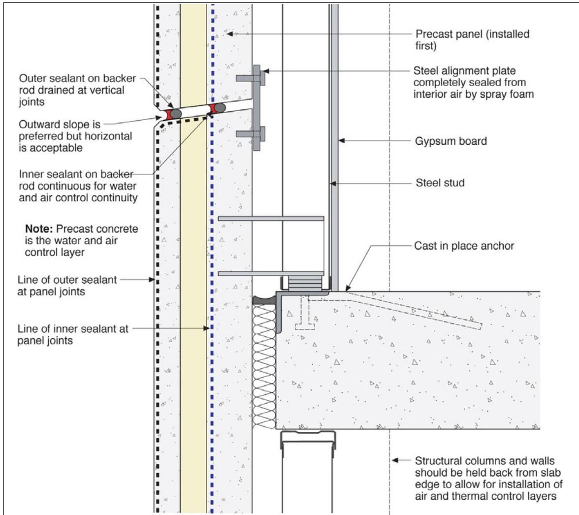
Figure 15: Section at floor of a high-performance double-wythe insulated precast concrete sandwich panel (CPCI 2013).
