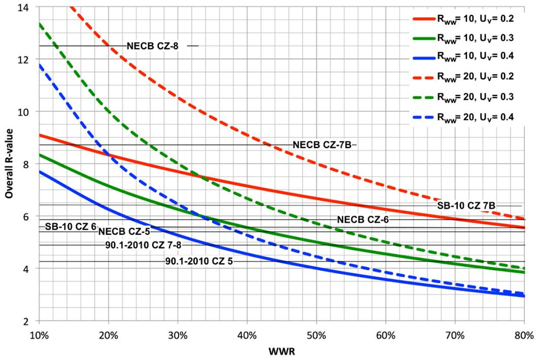
Figure 10: Combined impact of thermal performance of mass walls and windows and WWR (Note: CZ=climate zone,  $R_{ww}$  is whole-wall R-value, and  $U_v$  is window U-value).
