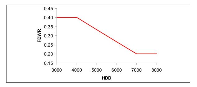
*Figure 3: Maximum fenestration-and-door-to-wall ratio (FDWR) under the NECB prescriptive approach.*
