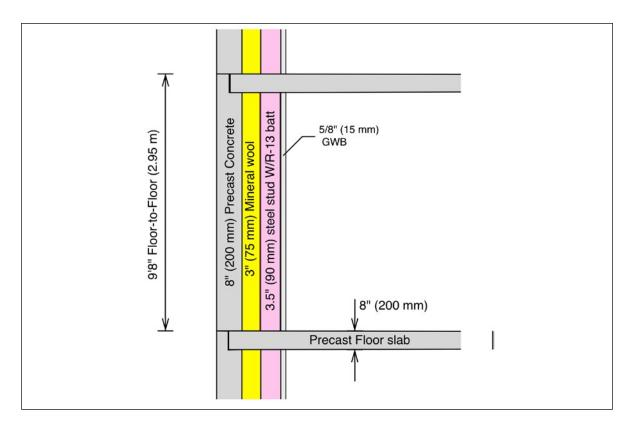
Figure 18: Example generic total precast whole wall.
