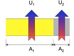
Figure 8: Parallel path heat flow.
