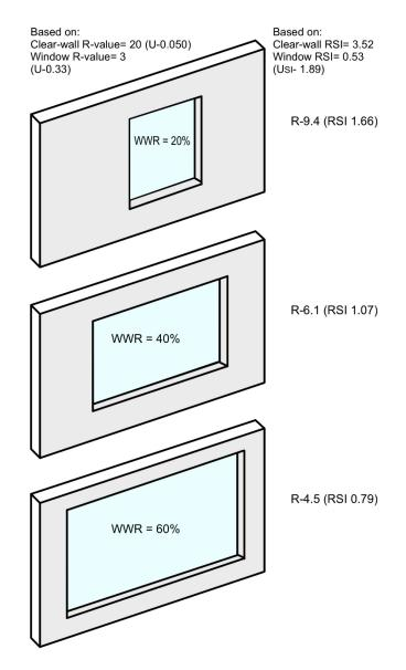
Figure 9: Impact of windows on overall enclosure R-value.
