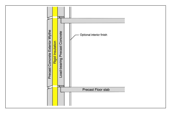
Figure 17: Double-wythe insulated "sandwich" total precast.
