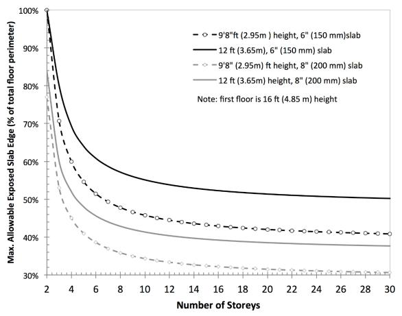
Figure 6: Maximum balcony perimeter per floor assuming 2% thermal bridging waiver.
