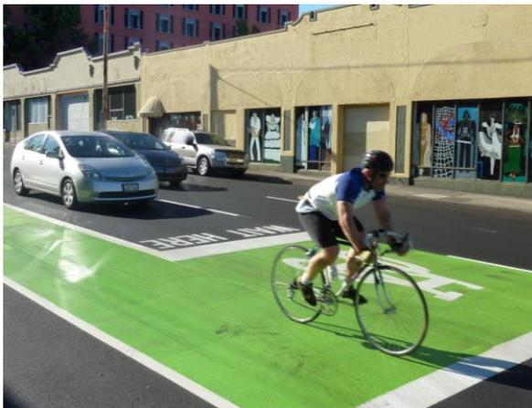
Bike Boxes are a new kind of street marking to help motorists and cyclists share the road. Bike boxes are used at intersections to designate a space for cyclists to wait in front of cars at a red light and then proceed first through the intersection when the light turns green. Once they clear the intersection they resume travelling in the bike lane.
