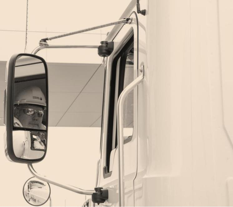
Having an effective mirror set-up and adjusting them properly can greatly reduce the potential of an on-road incident. This will also provide the driver with a huge amount of information by reducing the blind spots around the vehicle.
