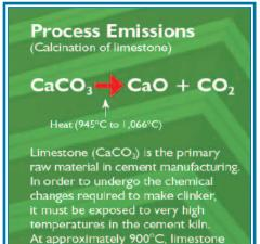
At approximately 900°C, limestone undergoes a fixed chemical reaction known as calcination (or decarbonation).  $CO_2$  is released as a direct by-product of this chemical reaction.
