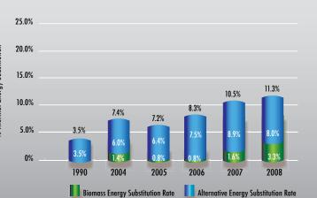
Cement kilns are well-suited for the use of alternative and renewable fuels, as the kiln process involves long residence times and high temperatures, ensuring complete destruction of organic compounds. As well, the remaining inorganic components (i.e. ashes) are integrated into the clinker product, rather than discarded as waste.
