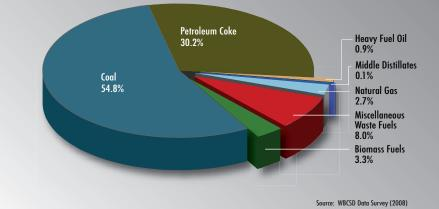
Canadian cement manufacturing operations are: construction and demolition wood wastes, municipal bio-solids, nonrecyclable plastics and textiles, recovered solvents, and discarded tires and the remaining tire fragments left over from tire recycling operations.
