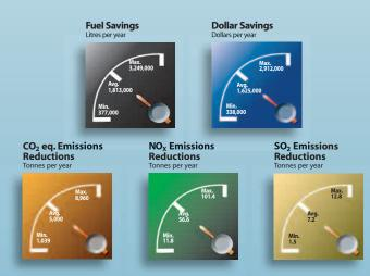
The range of potential fuel savings and reductions in emissions that will be achieved by trucks if a 100 km section of a major urban arterial highway in Canada were to be paved in concrete is presented here. It is assumed 1,095,000 heavy trucks travel on this section of roadway, based on 20,000 vehicles per day at 15% heavy truck traffic.
