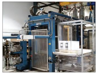
Newfoundland Styro uses this Kurtzs ICF machine to manufacture its insulated concrete forms
