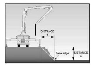
The One-to-One Rule: For every one foot of vertical drop, stay back from the base edge one foot. (Distance "B" must be equal to or greater than Distance "A")
